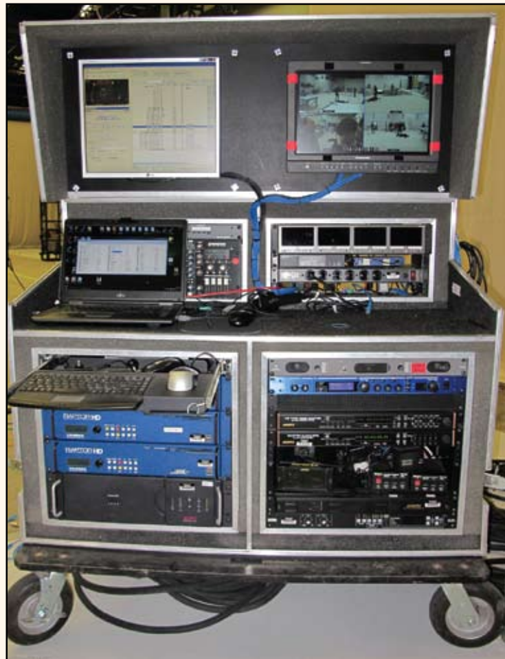
Front of one of the video assist carts for "Real Steel." Each day typically had nine cameras rolling — three Sony F35s and six Sony EX-3s — and video assist carts for all of them including Blackmagic Design mini-connectors and routers, including Blackmagic Smart Videohubs.
