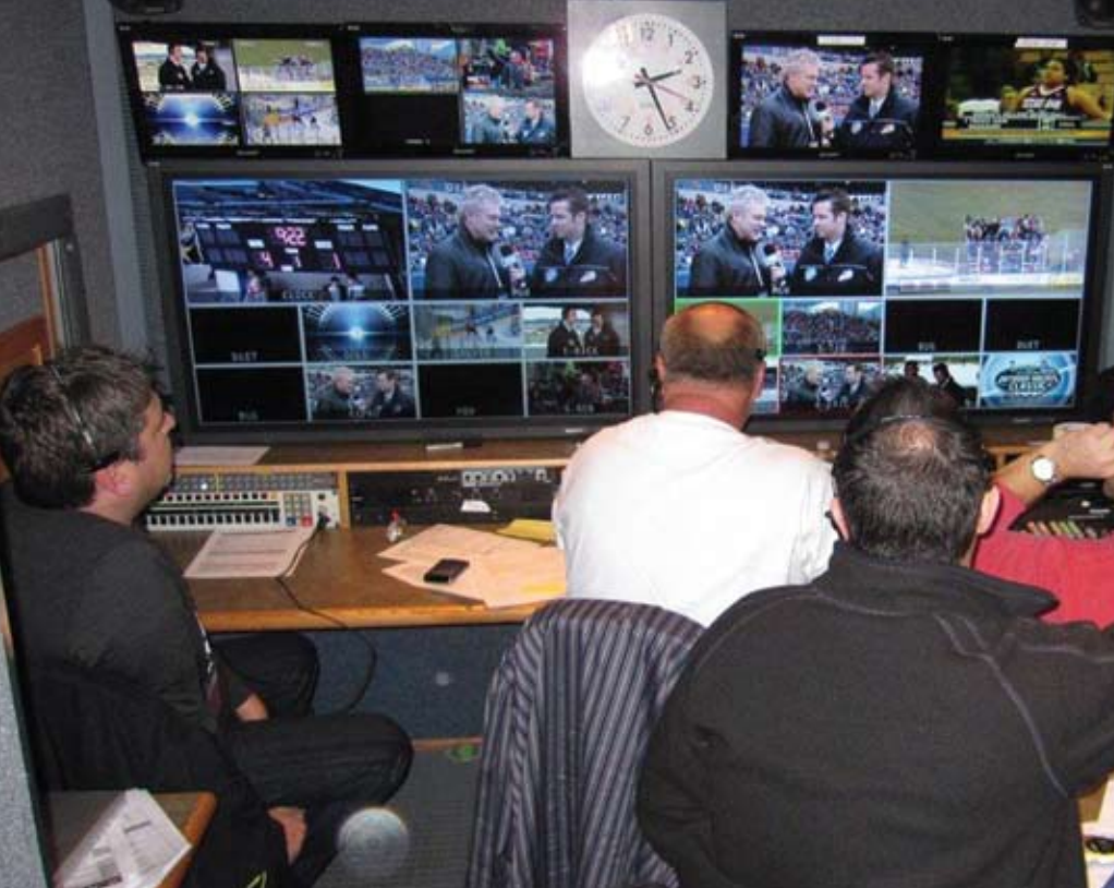
In the "DivaHD" production room, a small section of control area monitors with patch bays, all run through the 72x144 Broadcast Videohub.
